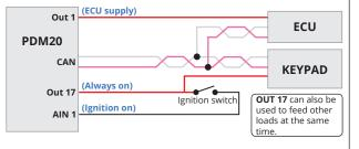
Keypad and ignition switch, low power mode support
